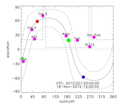
Figure 4. The graphic output of the IDL program, *radio\_coords*. The green dots indicate the Galactic center (large) and the Galactic anti-center (small). The red and blue dots point to galactic longitudes of 90° and 270° respectively. The sky coverage accessible to the antenna mount lies above the straight dashed lines. The difference between local time and GMT (UTC) is either 4 hours (in the summer) or 5 hours (in the winter).
